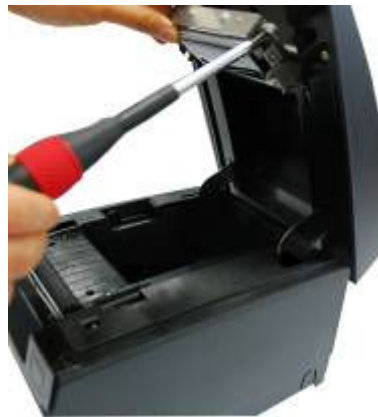
< Easy replacement of TPH / Auto-Cutter >
