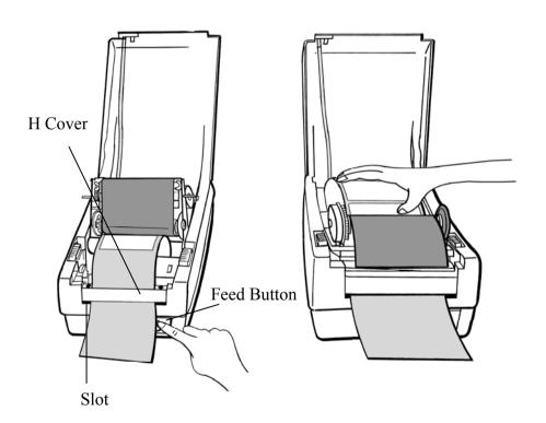
15. Close the top cover and turn on the printer or press the "FEED" button if the printer is already on.
