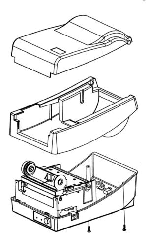
4. Remove the whole print head assembly by releasing the 4 screws at its feet.
