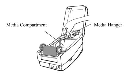
3. Load the media roll onto the hanger from left to right.
