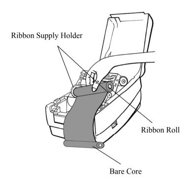
7. Put the print head module down and insert the bare core into the pick-up holder. (First snap in the left side, and then the right side.)
