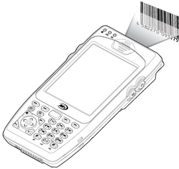
Make sure the laser beam covers whole barcode to read data properly.
