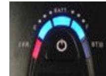
Error – Cover open (light-on) Out of paper (blinking)
