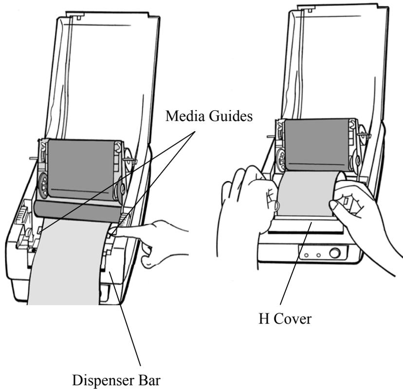
12. Press the "FEED" button for the label backing paper to come out from the slot under the H cover.
