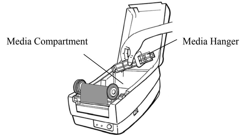
3. Load the media roll onto the hanger from left to right.
