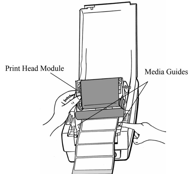
10. Put the print head module down and press down firmly until you hear a snap.
