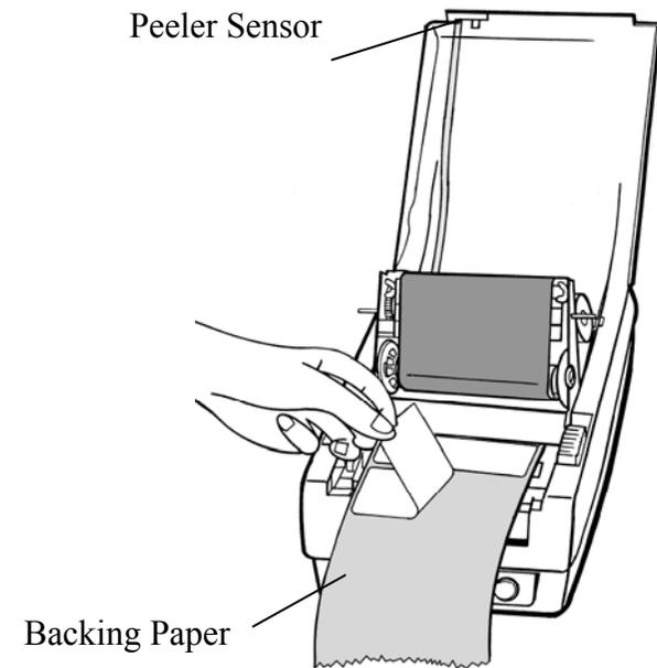
10. Trim the front edge of the label backing paper with scissors or a knife.
