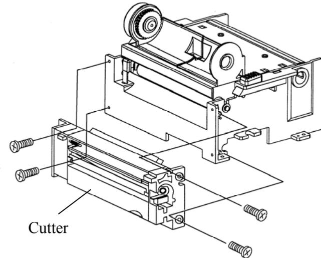
7. Plug the cutter's connector into the PCB's header connector (JP13).
