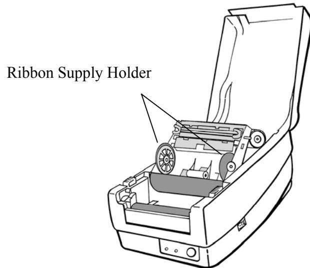
4. Unwrap the ribbon roll pack and separate the ribbon roll and the bare core.
