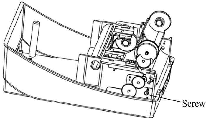
13. Unlatch the print head module. Hook the white roller on the brackets of the chassis, ensuring the long thinner end is on the left side.
