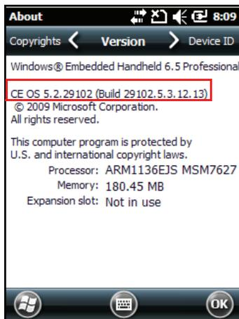
The second line lists the operating system version and the build number. The last part of the build number represents the AKU number. For example, *Build 29102.5.3.12.13* indicates that the device is running AKU version 5.3.12.13.
