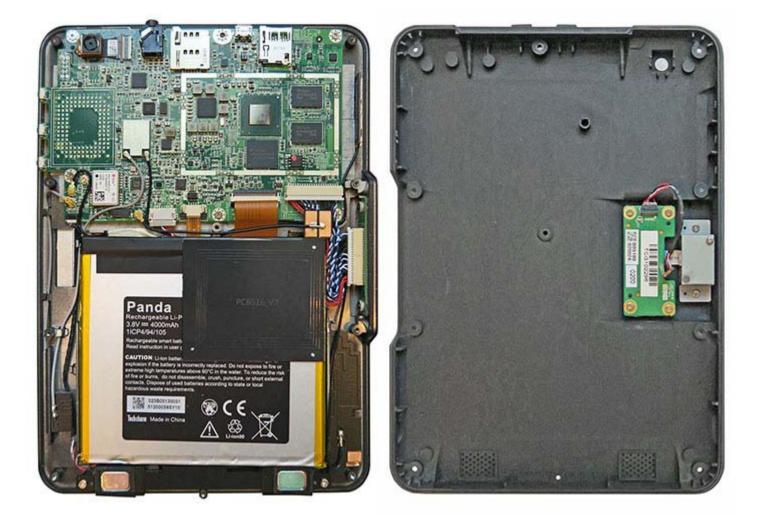
Prominently visible now is the large, but very thin, Lithium-Polymer battery. It's a 3.8 Volt, 4,000 mAh design that makes for 15.2 watt-hours. The battery sits loose in between two metal guides that are part of the overall aluminum front of the tablet. While not externally accessible, replacing the battery, which is plugged into the mother board, is therefore easy. The black rectangle on top of the battery is the NFC antenna.
