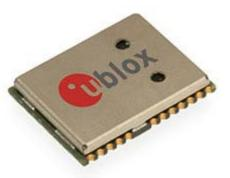
The only separate and distinctly visible module on the main board is a u-blox NEO-M8N GNSS module for positioning. One cool thing about the M8 is that it
