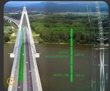
Valid speed detection at 600 m / 1968 ft, ANPR/LPR up to 150 m / 490 ft (nighttime up to 100 m / 328 ft).
