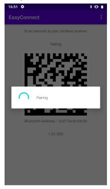
Once a scanner and an Android device is paired, no repairing is required unless the pairing information is cleaned.
