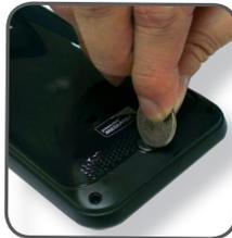
3. Detach and remove the battery chamber door.
