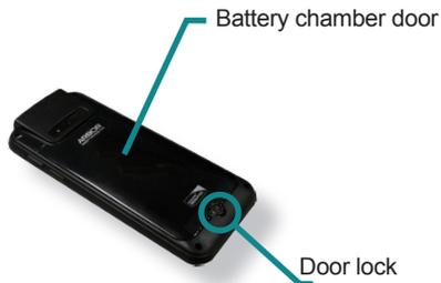
2. Use a coin to loosen the screw on the battery chamber door.
