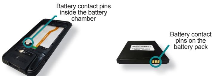
3. Place the battery into the battery chamber by an angle the contact pins can meet.
