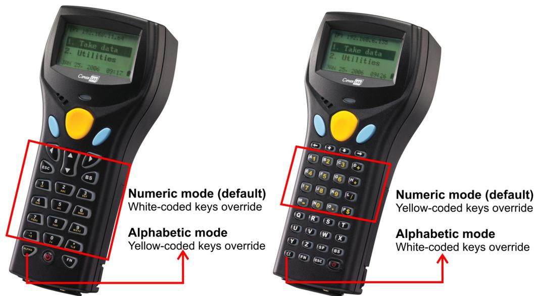
Figure 3: Keypad layout - 24-key (left), 39-key (right)
