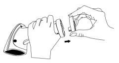
3. Pinch the tape at the top of the battery and pull the battery out.
