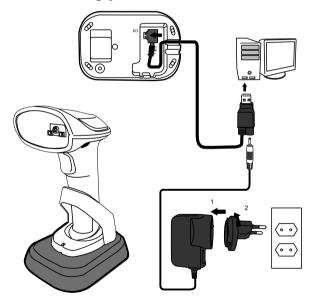
Connect the USB or the RS-232 cable to your cradle. Lay the cable into the notch on the cradle edge. Connect the USB or the RS-232 cable to your computer.
