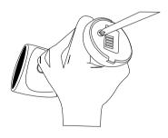
2. Remove the battery cap.
