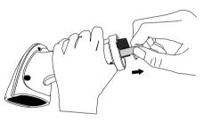
4. Insert the new battery into your scanner in the direction of the arrow printed on the battery.
