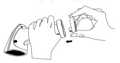
6. Tighten the screw to secure the cap.
